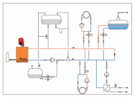
INTEC® plants allow the connection of different consumers The main components of the INTEC® heater are manufactured in Germany by INTEC Rohrtechnik GmbH providing the highest possible quality level
